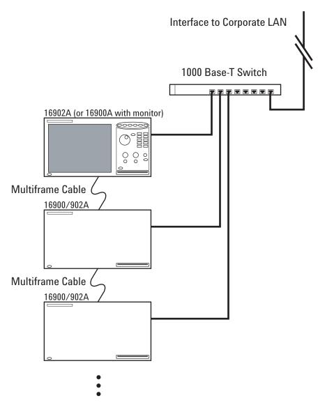
In the simple 1000 Base-T multiframe configuration, all of the frames are connected to the network using their 1000 Base-T LAN port.
