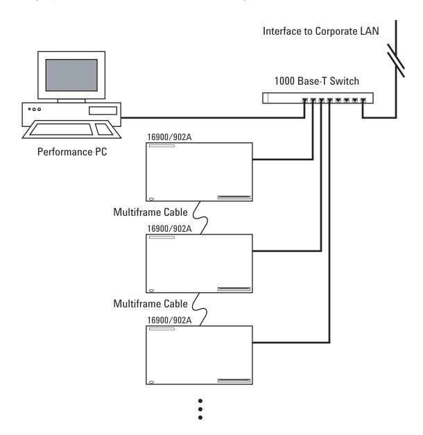
In the performance multiframe configuration, you run the *Agilent Logic Analyzer* application on a high-performance PC or server. This is useful if you trying to maximize multiframe logic analysis system performance.
