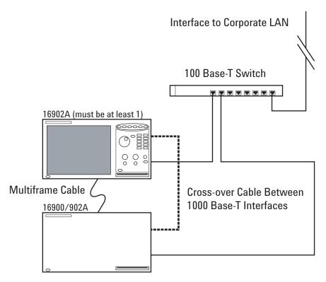
When you have only two frames in the simple 100 Base-T multiframe configuration (see page 59), you can gain performance by connecting a crossover cable between the frames' 1000 Base-T ports and configuring these ports with static IP addresses.
