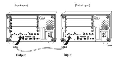
One frame's output is connected to the next frame's input, and so on.
