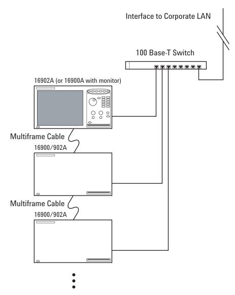
In the simple 100 Base-T multiframe configuration, all of the frames are connected to the network using their 100 Base-T LAN port.
