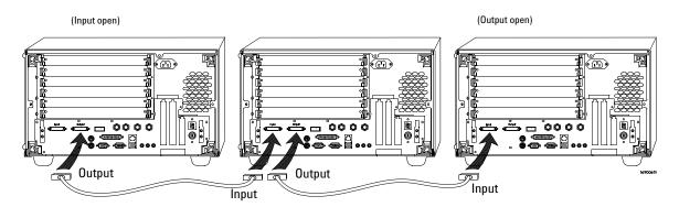
One frame's output is connected to the next frame's input. Connect multiple frames in sequence with the final frame having no output connected.
